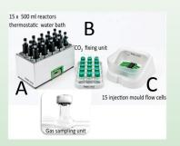
Figure 1: AMPTSII for biomethane potential assays. The AMPTSII can be divided into three units: A, B and C. Unit A is the sample incubation unit, with controlled stirring possibilities and a thermostatic water bath. The gas released from unit A is measured using a wet flow-measuring device with a multi-flow cell arrangement. This measuring device works according to the principles of liquid displacement; a digital pulse is generated when a defined volume of gas flows through the unit.
