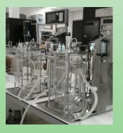
Figure 4: Two Infors 13 liter Labscale Bioreactors: Both bioreactors are a continuous stirring type reactor (CSTR) with an reactor volume of 10 litres. The bioractors are fed on daily basis with (= ~7% (ODM) maize slurry) with an OLR of 1,25 kg ODM\*m³day¹. The hydraulic retention time was kept at 40 days. The default process temperature was 35 °C. The content of the reactor was stirred at 50 mm.
